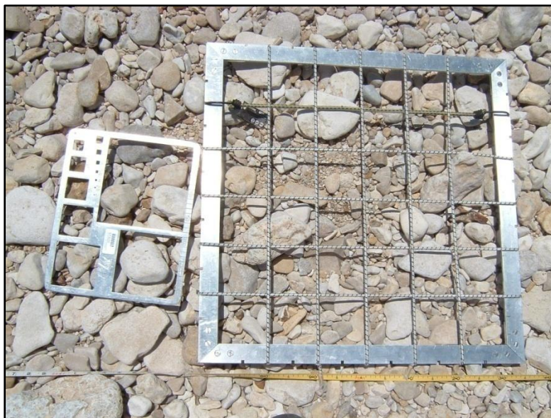
Figure 4.4. Equipment used for modified Wolman pebble count procedure on cobble-to gravel-sized bed material.
