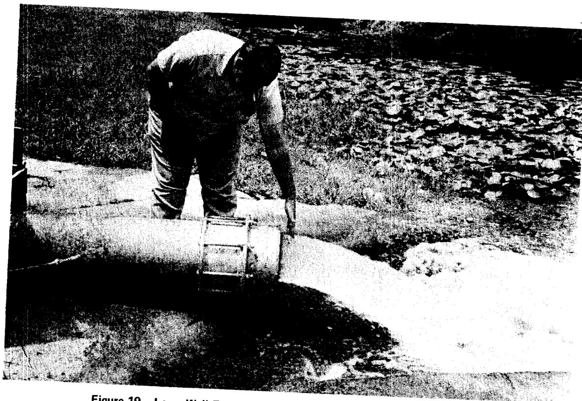
Figure 19.—Large Well Flowing From the Edwards (Balcones Fault Zone) Aquifer at Fort Sam Houston in San Antonio (Courtesy of U.S. Department of Agriculture, Soil Conservation Service)
