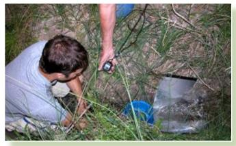
Measuring springflow with a bucket and stopwatch
