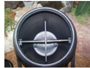
Center cross T used to break up composting material each time the composter barrel is turned
