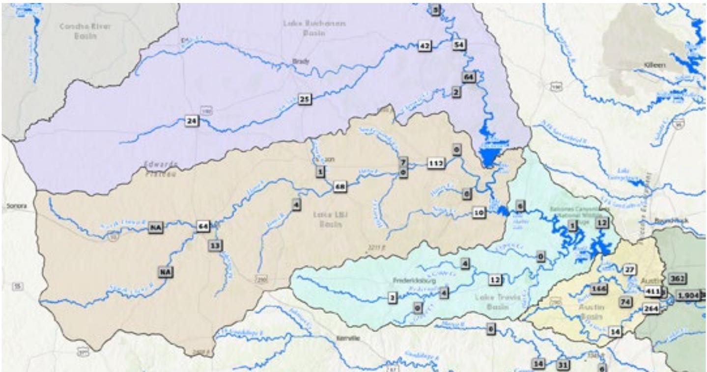
Lower Colorado River Authority’s Hydromet is a system of more than 275 automated river and weather gauges throughout the lower Colorado River basin in Texas. The website displays gauges maintained by the City of Austin and USGS. The Hydromet provides near-real-time data on stream-flow, river stage, rainfall totals, temperature and humidity. <https://hydromet.lcra.org>
